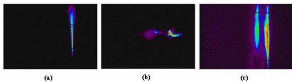
Figure 3: Raw energy spectrums of double-bunch e-beam. Energy dispersion increases to the left. (a) Before the chicane and without compression. Energy spread is ~4% FWHM. (b) At the high-energy slit located downstream of the chicane. (c) At the spectrometer at the end of the beamline.
