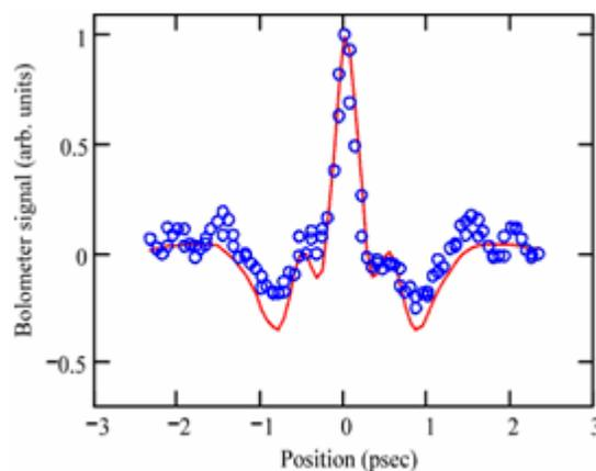
Figure 5: Example of raw data from CTR interferometer (circles) and the curve fits to the data (solid line) calculated from the autocorrelation integral.
