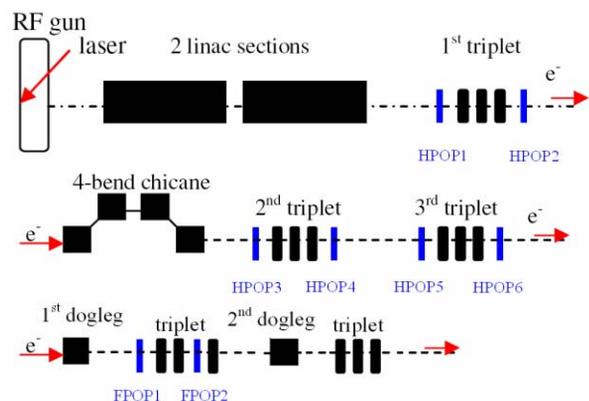
Figure 1: Schematic of the ATF H-Line/dogleg system; the beam bends in the vertical (y) plane in the chicane.
