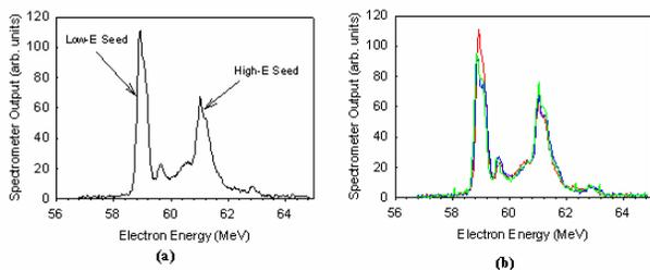
Figure 4: Energy spectrums of double-bunch e-beam. (a) Typical single shot spectrum for the case when both bunches have comparable charge. (b) Three spectrums taken many minutes apart demonstrating stability of the double-bunch formation process.
