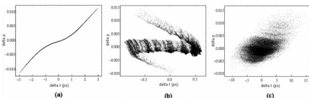
Fig. 6: Longitudinal phase space from the program elegant of the chicane/dogleg system. (a) Momentum-time plot of electrons entering the chicane. (b) Momentum-time plot of electrons leaving the chicane. (c) Momentum-time plot of electrons at exit of 2<sup>nd</sup> dogleg.
