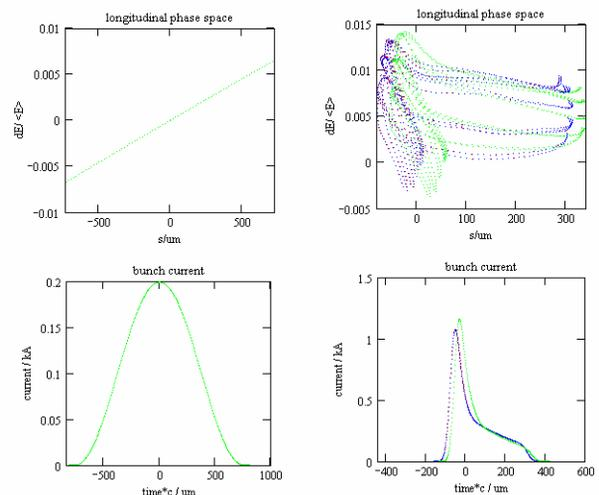
Fig. 7: Longitudinal phase space and bunch current distribution given by the code CSRTrack with the 1D projected method (green points), the 2D Green's function method (blue points) and the 3D convolution method (red points) before (left two plots, blue and red behind green) and after the bunch compressor chicane (right two plots, red behind blue).
