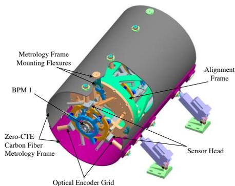
Figure 2: The NanoBPM experiment including the metrology system.
