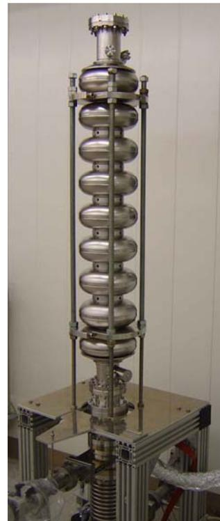
Figure 1: TESLA cavity during high pressure water rinsing at ACCEL. The high pressure water rinsing system is installed in a class 100 clean room.
