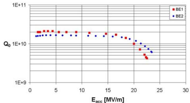
Figure 4: Test results of cavity BE1 and BE2. Fields above 20 MV/m with  $Q$  higher than  $1 \cdot 10^{10}$  were reached. At the highest fields some field emission was observed. Both cavities were checked for Q-disease and proven to be Q-disease free.
