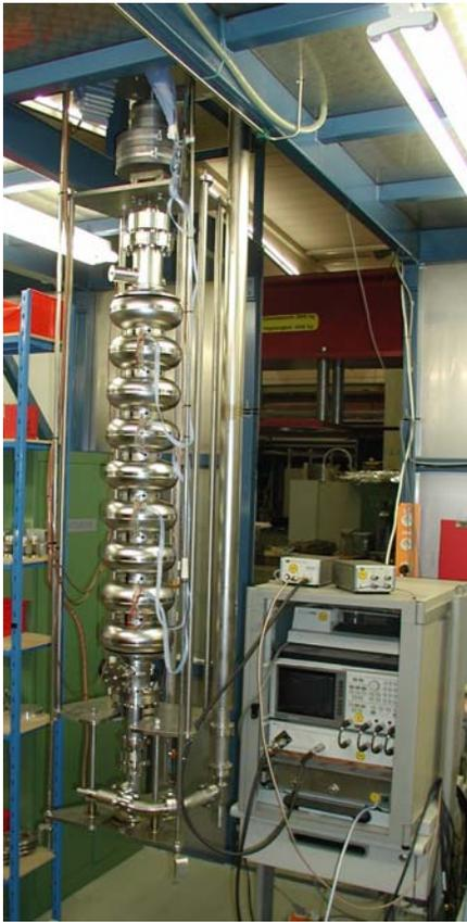
Figure 2: TESLA cavity assembled to the vertical test stand at DESY
