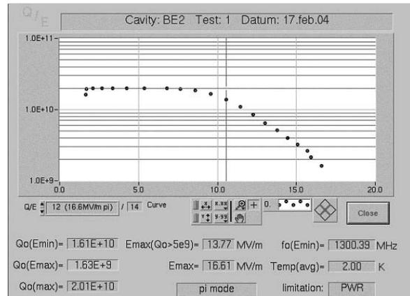
Figure 3: First test of cavity BE2. Field emission limited the cavity to about 16.8 MV/m.
