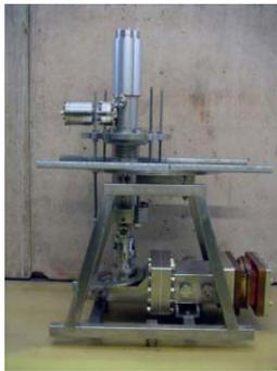
Figure 2: Coupler stand used for warm coupler tests.
