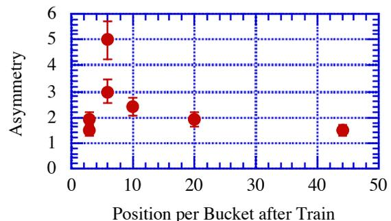
Figure 5: Asymmetry in the spectrum as a function of the bunch location after colliding bunches. One bucket corresponds to 2 ns.
