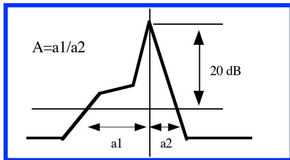
Figure 3: Definition of asymmetry in the spectrum.
