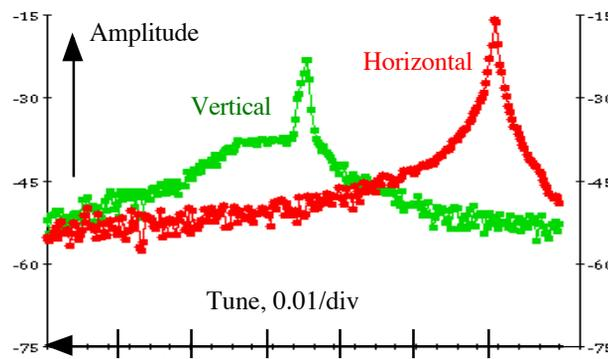
Figure 1: Tune spectra of a pilot bunch observed at the HER under normal colliding operations; the horizontal scale is the tune going right to left with a full scale of 0.07. Vertical is the amplitude with log-scale in dB. The red curve is the horizontal spectrum with a fractional tune of 0.511 and green is vertical with a tune of 0.582.
