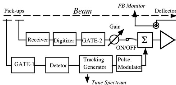
Figure 2: Schematic diagram of a gated tune monitor and a transverse feedback system.
