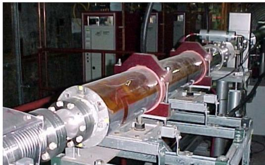
Figure 2: Pulsed quadrupole in the RHIC tunnel in a section common to both beams.
