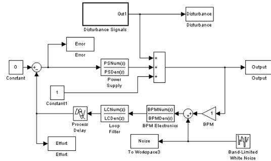
Figure 6: Position loop MatLab model.
