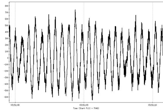
Figure 3: 10 Hz beam oscillations as detected by the DX BPM.
