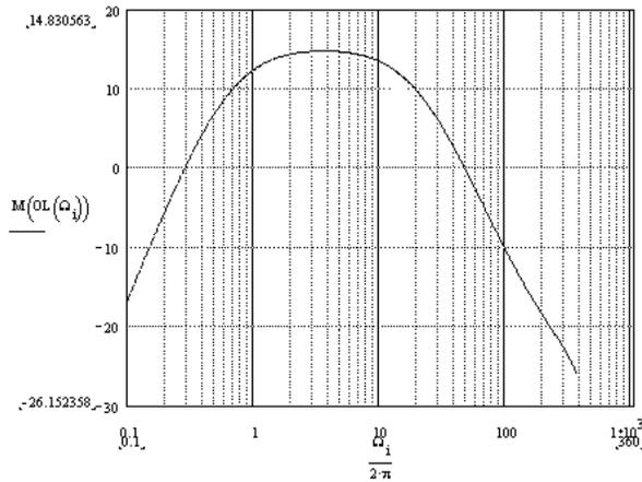
Figure 5: Open-loop response of the position loop.
