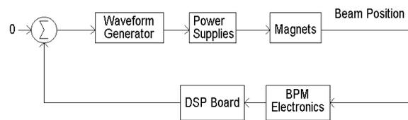
Figure 4: Hardware block diagram.
