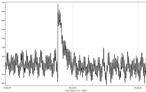
Figure 2: Signal shift due to auto gain bit change.
