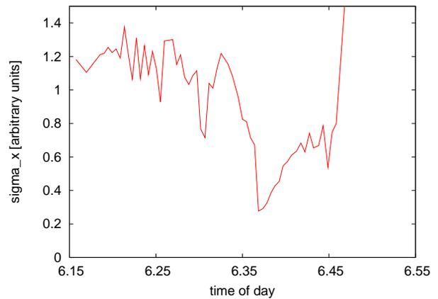
Figure 4: Measured horizontal rms beam jitter in the frequency range from 8.5 Hz to 14.5 Hz when the helium circulators in both rings were turned off.
