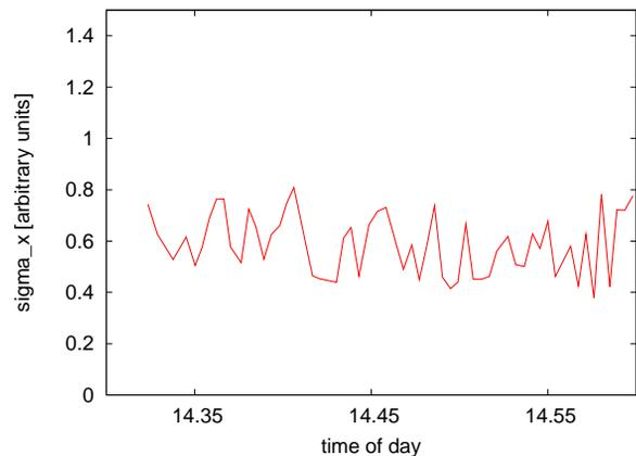
Figure 5: Example of measured horizontal rms beam jitter in the frequency range from 8.5 Hz to 14.5 Hz during regular beam operations in FY05.
