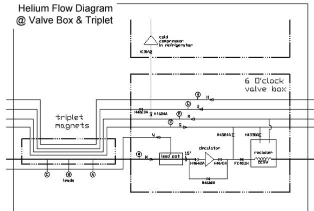
Figure 2: Flow diagram of the RHIC triplet cryostat and the associated valve box at the 6 o'clock location.
