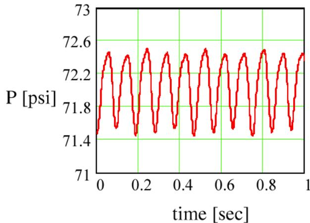
Figure 3: Measured helium pressure  $P$  in the magnet line “M” vs. time. The frequency of the observed pressure oscillation is 10.7 Hz.
