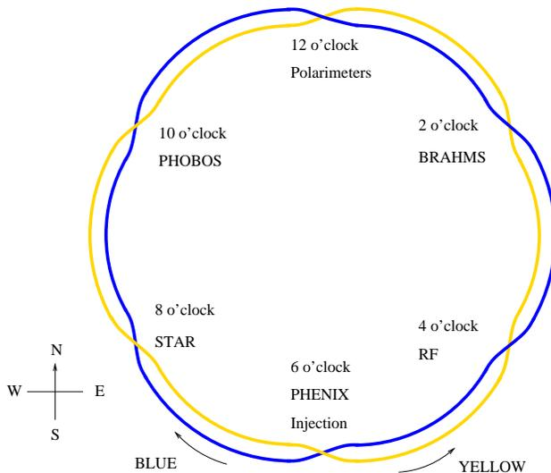
Figure 1: Schematic overview of the RHIC collider with its six interaction regions.
