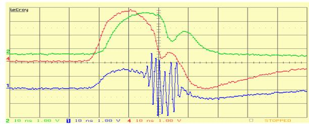
Figure 4: Fast instability observed in the CERN PS near transition ( $\sim 6$  GeV total energy) in 2000. Single-turn signals from a wide-band pick-up. From top to bottom:  $\Sigma$ ,  $\Delta x$ , and  $\Delta y$ . Time scale: 10 ns/div. The head of the bunch is stable and only the tail is unstable in the vertical plane. The particles lost at the tail of the bunch can be seen from the hollow in the bunch profile.
