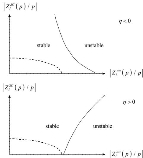
Figure 5: Stability diagram for the LMC instability below and above transition respectively for a proton bunch. The Keil-Schnell circle is represented by the dashed curve.
