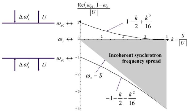
Figure 7: Evolution of the coherent synchrotron frequency for the dipole mode with respect to the incoherent frequency spread.
