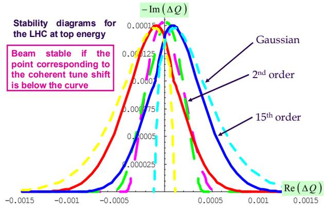
Figure 6: Stability diagrams (positive and negative detunings) for the LHC at top energy (7 TeV) with maximum available octupole strength, for the 2<sup>nd</sup> order (dashed curves), the 15<sup>th</sup> order (full curves), and the Gaussian (dotted curves) distribution.
