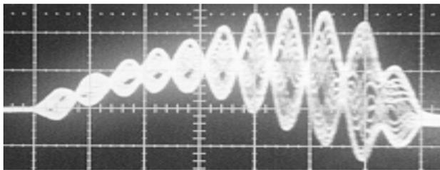
Figure 3: Signal from a radial beam position monitor during 20 consecutive turns observed in the CERN PS at 1.4 GeV kinetic energy in 1999. Time scale: 20 ns/div.
