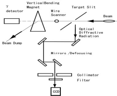
Figure 1: A Schematic Diagram of the Experiment.
