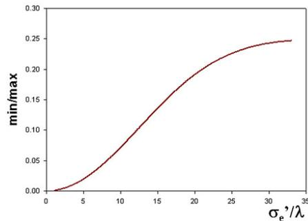
Figure 5: min/max ODR photon yield ratio as a function of the transverse beam size with the curved disphased target.
