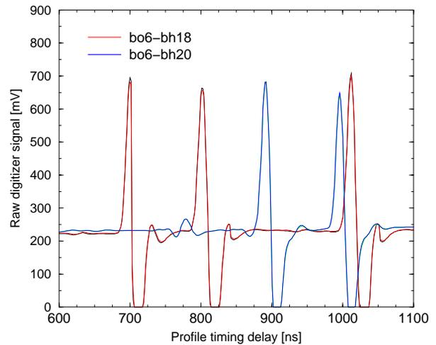
Figure 2: Profile timing scans for BPMs bo6-bh18 and bo6-bh20, with 105 ns bunch spacing. The vertical axis is digitizer voltage from each BPM stripline.
