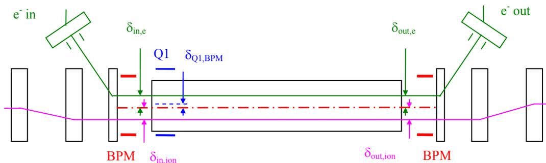
Figure 1: A simplified schematic of the measurement setup, showing only the first alignment quadrupole.
