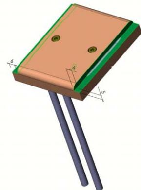
Figure 4: A tuning plate with cooling pipes.
