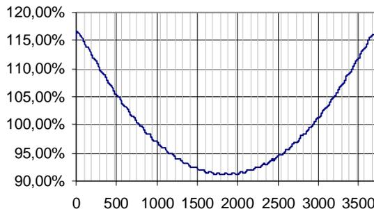
Figure 2: Simulation result of the flatness calculation in a simple 40 stem RFQ design.
