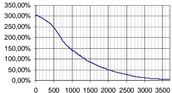
Figure 3: Simulation result of the flatness calculation in a 40 stem RFQ design with varying aperture and electrode modulation.
