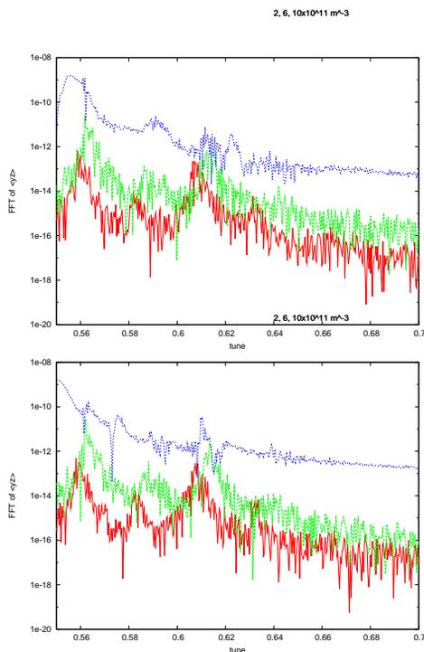
Figure 5: Frequency spectra for the correlation function ( $\langle\langle yz \rangle\rangle$ ) obtained by a simulation. Top and bottom pictures depict spectra for damping time of 50 and 200 turns, respectively. Three lines, red, green and blue, corresponds electron cloud densities, 2, 4 and  $6 \times 10^{11} \text{ m}^{-3}$ , respectively.
