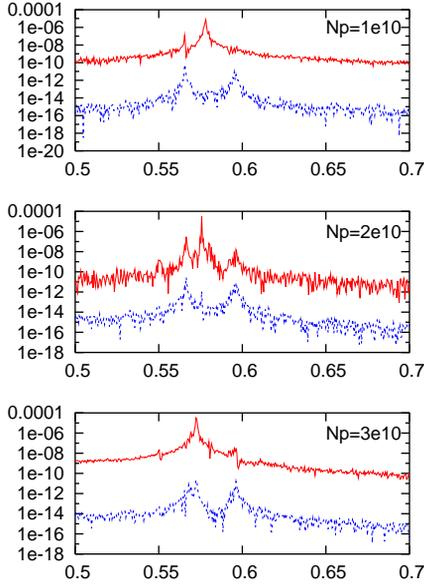
Figure 2: Typical frequency spectra for an ordinary wake,  $W(z) = az$  (simulation with  $\nu_\beta = 0.58$ ). Beam intensity are increased for lower picture. Red and blue lines are frequency spectra for  $\langle y \rangle$  and  $\langle yz \rangle$  motions, respectively.
