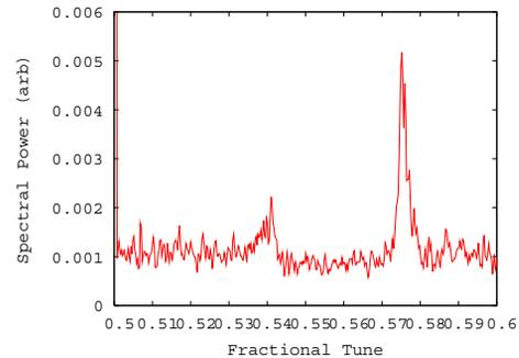
Figure 1: Typical synchro-beta sideband spectrum observed above the threshold of the beam size blow-up due to electron cloud (measurement). The vertical betatron tune is set  $\approx 0.535$  in this measurement.
