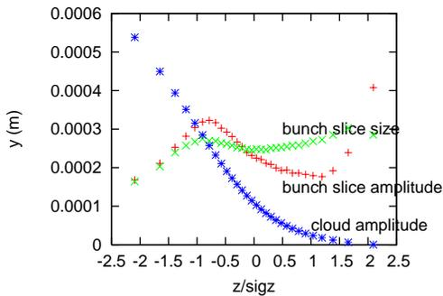
Figure 3: Typical bunch and electron cloud profile obtained by a simulation.
