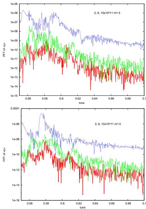
Figure 4: Frequency spectra for vertical averaged position ( $\langle\langle y \rangle\rangle$ ) obtained by a simulation. Top and bottom pictures depict spectra for damping time of 50 and 200 turns, respectively. Three lines, red, green and blue, corresponds electron cloud densities, 2, 4 and  $6 \times 10^{11} \text{ m}^{-3}$ , respectively.
