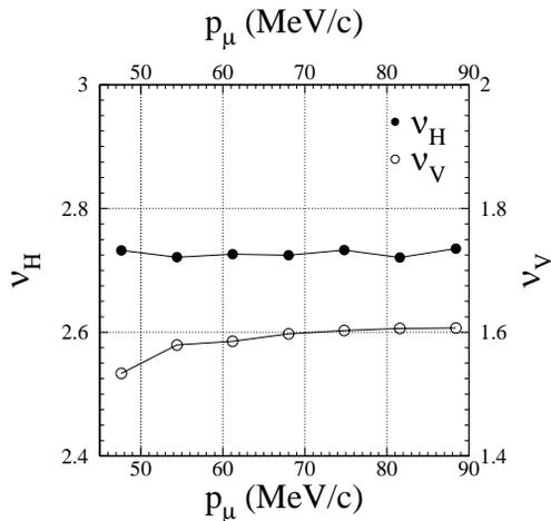
Figure 4: Horizontal and vertical betatron tunes as a function of muon momenta, showing zero-chromaticity for the PRISM FFAG ring.
