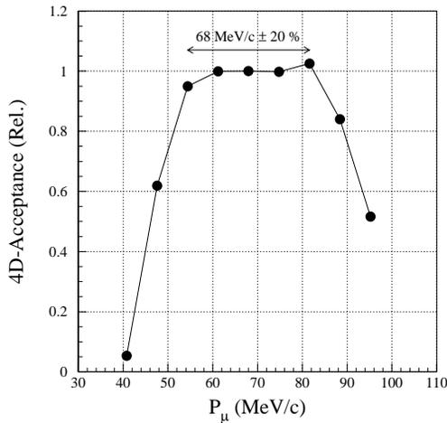
Figure 3: Momentum acceptance of the PRISM FFAG ring.
