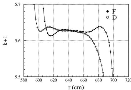
Figure 8: The  $k + 1$  values of the field integral "BL" on the median plane.
