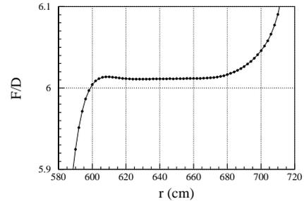
Figure 9: The F/D ratio of the field integral "BL" on the median plane.
