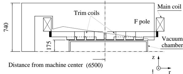
Figure 6: Side view of one F magnet for the PRISM FFAG ring.
