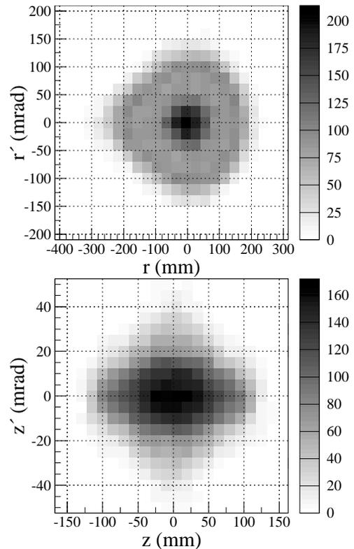
Figure 2: Horizontal (top) and vertical (bottom) acceptance of the PRISM FFAG ring. The gray scale represents the intensities.
