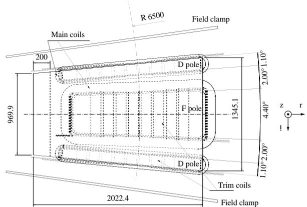
Figure 5: Plane view of one DFD magnets for the PRISM FFAG ring.
