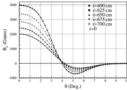
Figure 7: Azimuthal distribution of the magnetic field of the PRISM FFAG ring.
