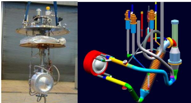
Figure 4: Two LH<sub>2</sub> absorber prototypes, convection type, internal heat exchange (left) and forced-flow, external heat exchange (right).
