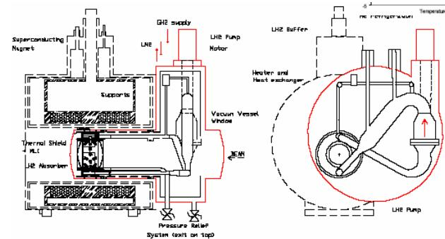
Figure 6: LH<sub>2</sub> forced-flow, external heat exchange prototype, shown inside a cryostat, inserted into the bore of the MTA solenoidal magnet sideview(left) and beam view (right).
