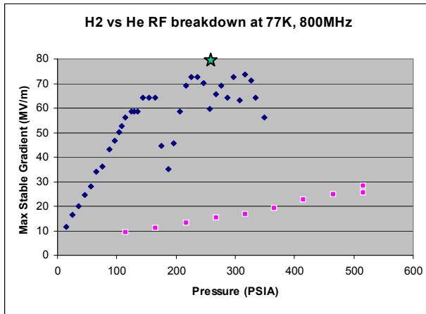
Figure 7: Paschen curve measurements for hydrogen (diamonds) and helium (squares). After a period of conditioning, a maximum gradient of 80MV/m was achieved (star) in GH<sub>2</sub>.
