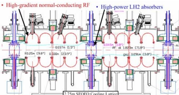
Figure 2: Cooling channel from Neutrino Factory Study II.
