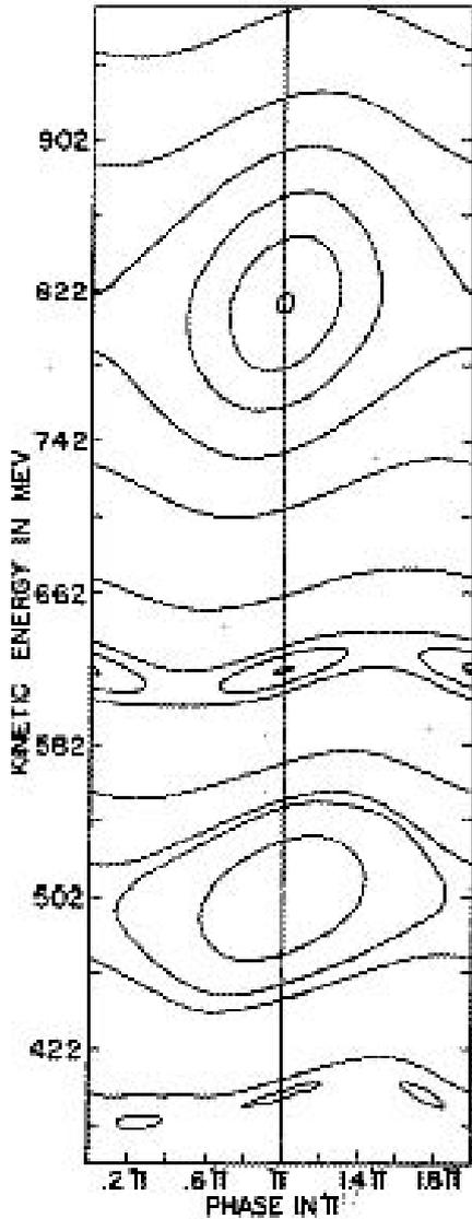
Figure 5: Numerical Simulation of rf Acceleration
