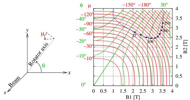
Figure 2: The helical rotators rotate the spin by an angle  $\mu$  about an axis transverse to the beam as shown in the left diagram. The plot on the right shows contours of  $\mu$  and  $\theta$ , the angle of the rotation axis from the  $x$ -axis for various settings of fields in the inner and outer pairs of helices.
