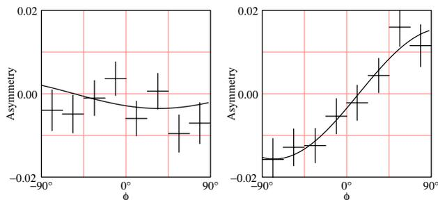
Figure 7: PHENIX asymmetries measured after correcting the polarities of the power supplies. Both sets of rotators were set to the currents:  $I_{in} = 184$  A and  $I_{out} = 221$  A. The negligible asymmetry in the Blue ring (left plot) is consistent with longitudinal polarization at PHENIX. The Yellow ring measurement (right plot) still shows a sizable vertical component due to the weak snake as discussed in the text.
