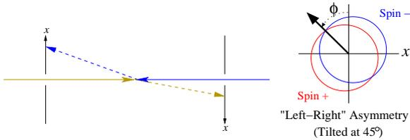
Figure 3: Left: Layout of the local PHENIX polarimeters around the interaction region. The  $y$ -axis (vertical) is out of the page; each local polarimeter has a right-handed Cartesian system with  $z$ -axis pointing along the corresponding beam direction. Right: definition of the left-right asymmetry indicating a polarization tipped away from the vertical axis by an angle  $\phi$ .
