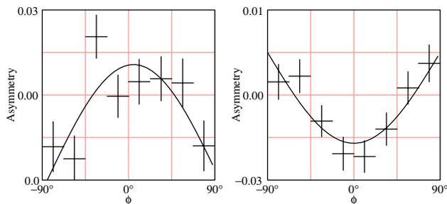
Figure 6: PHENIX asymmetries measured after first turning on the rotators at PHENIX with reversed currents ( $I_{in} = -184$  A and  $I_{out} = -221$  A): left is for the Blue ring, and right is for the Yellow ring.
