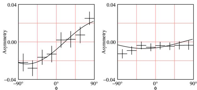
Figure 8: Further PHENIX asymmetries for the Yellow ring with rotator adjustments. A setting of  $I_{out} = 198$  A and  $I_{in} = 229$  A shown at left increased the transverse component. At right the setting with currents  $I_{out} = 244$  A and  $I_{in} = 138$  A eliminated the transverse component.
