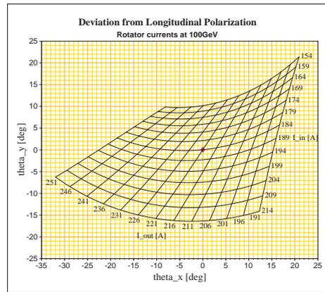
Figure 5: Sensitivity of polarization direction to rotator settings at 100 GeV. The angles  $\theta_x$  and  $\theta_y$  are defined in terms of the polarization components by the equations  $\tan \theta_x = P_x/P_z$  for horizontal and  $\tan \theta_y = P_y/P_z$  for vertical.
