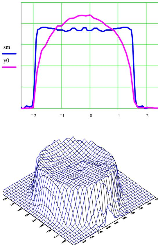
Fig.7: 1-D and 2-D beam profiles (magenta-signal from the wire, blue-restored beam profile).  $I_{\text{peak}}=2\text{A}$ .
