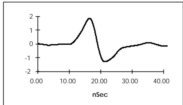
Fig.2: Typical BPM doublet signal
