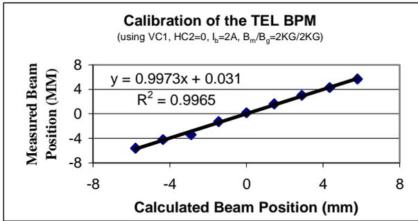
Fig.3: The linearity measurement of the BPM.
