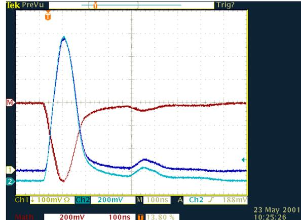
Fig.5: The signal from electron beam BPM system (The two blue traces are the signals from different plate of the same pair of pickup electrodes; the red trace is the difference signal of them.)
