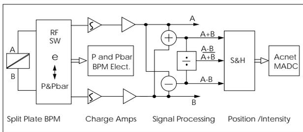
Fig.4: Diagram of electron BPM
