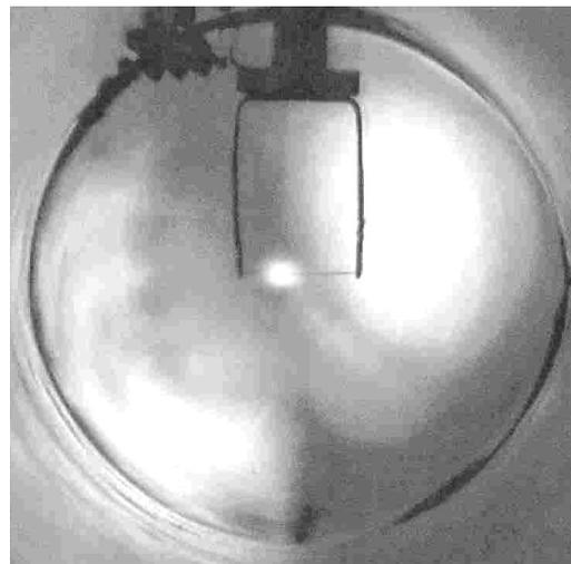
Fig.6: Shining electron beam on the scanning wire.
