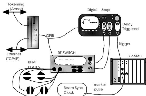
Fig.1: Proton BPM configuration.
