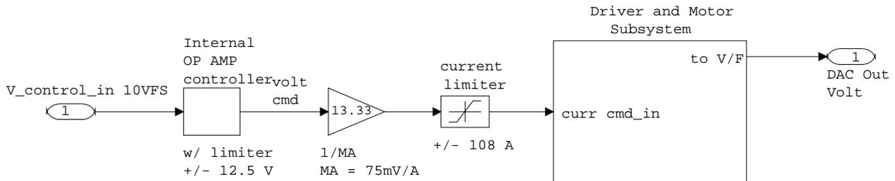
Figure 2. Top-level Simulink/MATLAB model of the PHAROS T-zero chopper.
