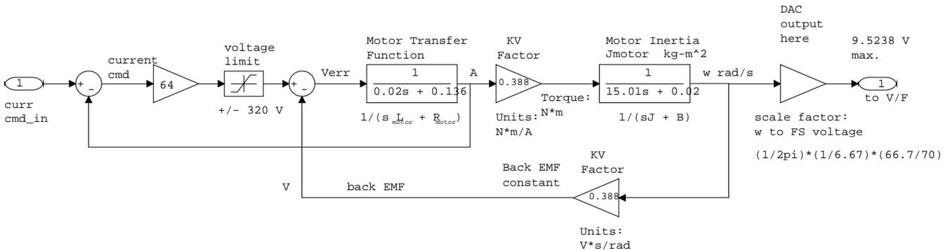
Figure 3. Expanded view of the driver and motor subsystem.
