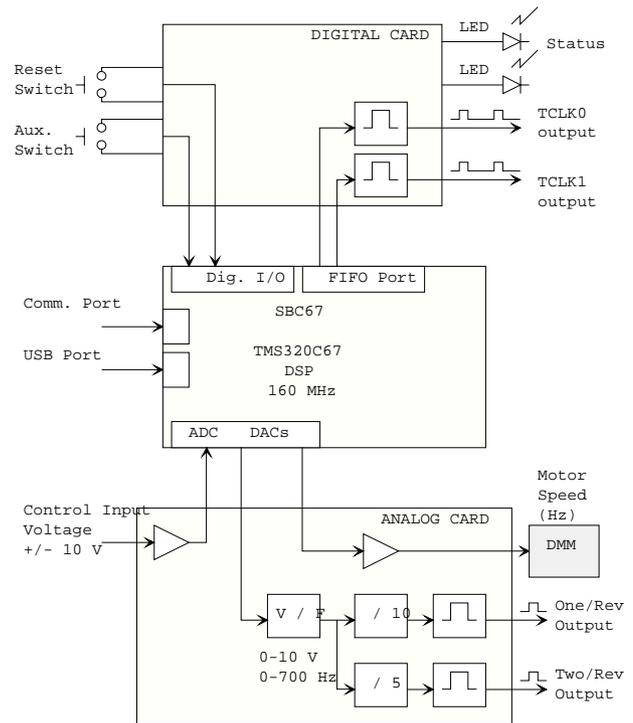
Figure 1. Block diagram of the simulator chassis.
