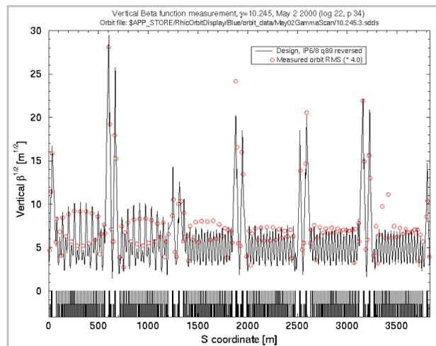
Figure 2: Measured -o- and predicted  $\beta_y$  betatron function in the vertical plane.
