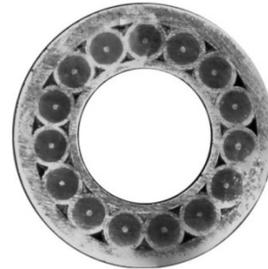
Figure 1: Cross-section of cable in conduit design.
