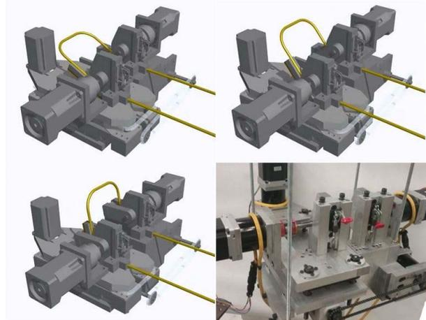
Figure 5: Bender for 90 degree bend.
