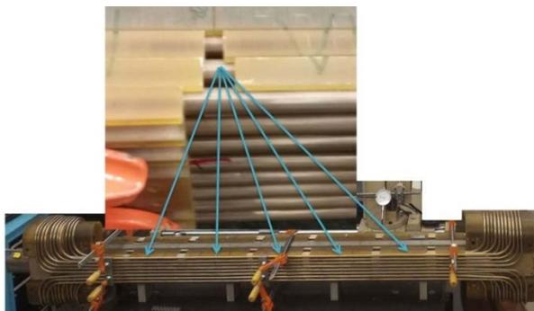
Figure 7: Locations along body of magnet to find cable placement and an example measurement.
