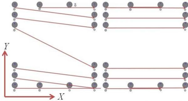
Figure 3: The left picture shows the transition end where the cables are transitioning from one level to another and the right shows the non-transition end. This is just for layer one.
