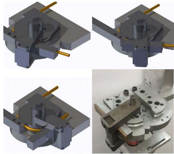
Figure 4: Bender for 180 degree bend.
