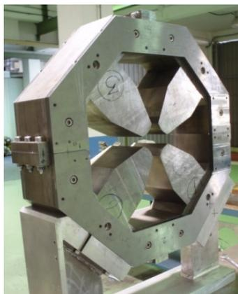
Figure 3: Magnetic yoke quadrants assembled and mounted in the magnet base support.
