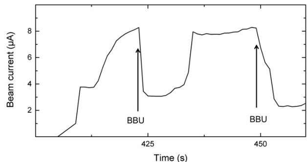
Figure 4: Beam current measured at a Faraday cup after the electrons were twice recirculated (three linac passes) with injection energy of 3.5 MeV. Skew quadrupoles in the first recirculation loop were used to mix the transverse phase advance which resulted in an increased threshold current of 8.2  $\mu\text{A}$ .
