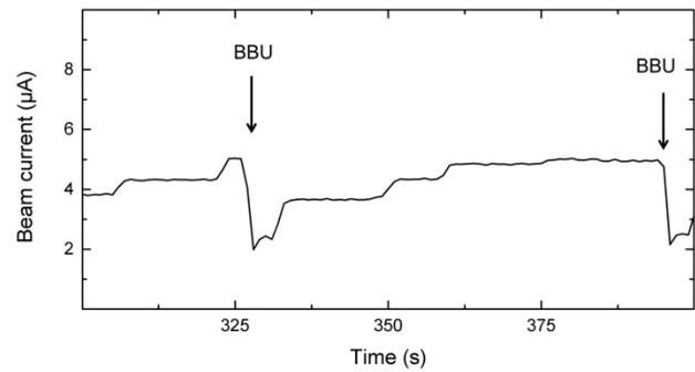
Figure 3: Beam current measured at a Faraday cup after the electrons were twice recirculated (three linac passes) with injection energy of 3.5 MeV. Turning up the current the beam was lost due to BBU at 5  $\mu\text{A}$ .
