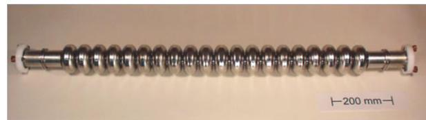
Figure 2: Picture of a S-DALINAC 20 cell cavity.
