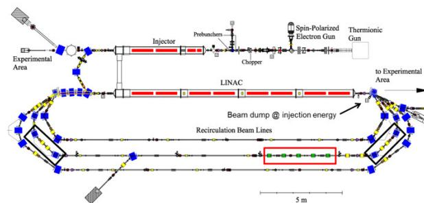
Figure 5: Floorplan of the S-DALINAC in 2016. A third recirculation loop has been installed between the two existing ones [2]. The dipole magnets inside the black rectangles will be movable to allow the necessary shift of the path length in order to run the accelerator as a single- or double-turn ERL. Five skew quadrupole magnets were installed (red box) to mix the transverse phase space advance.
