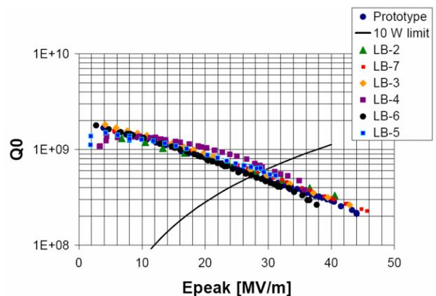
Figure 2: Test results of the halfwave resonators produced for the SARAF linac.
