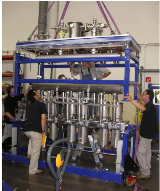
Figure 3: Intermediate assembly step of the prototype superconducting module. The completed string of six cavities and three solenoids is attached to the top plate
