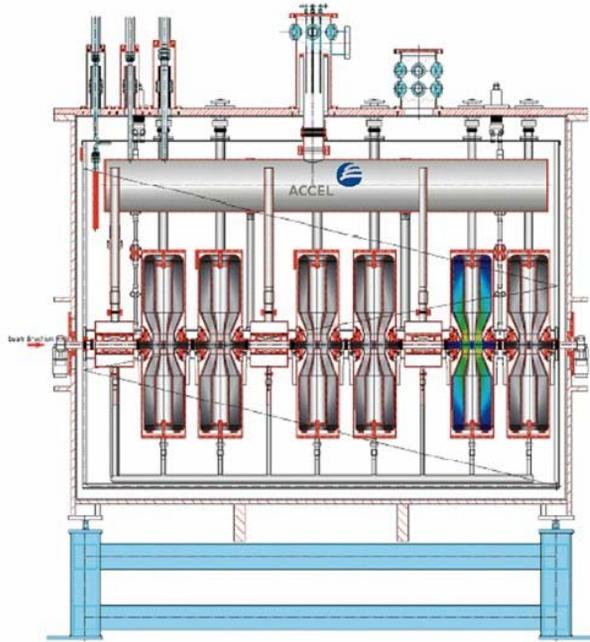
Figure 1: Prototype superconducting module containing six superconducting halfwave resonators ( $\beta=0.09$ ) and three superconducting solenoids
