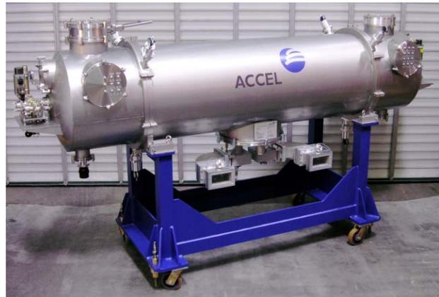
Figure 7: SRF module for 4GLS after successful cold test at ACCEL and ready to ship.
