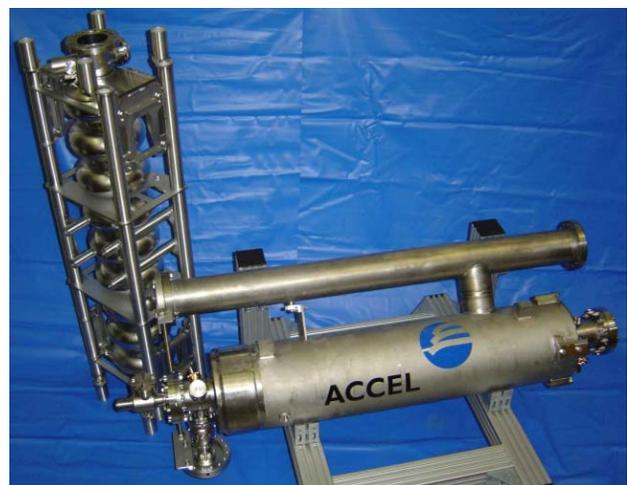
Figure 1: TESLA cavities produced at ACCEL; for one cavity the helium vessel is already welded and the high power coupler and the HOM antennas are assembled inside the clean room after preparation for horizontal test. The other cavity is mounted inside a transport frame.
