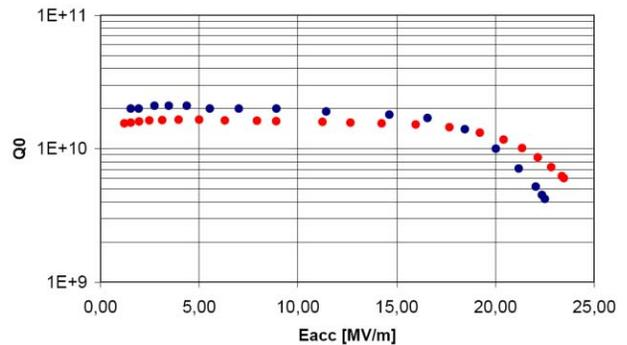
Figure 4: Vertical test result of TESLA cavities produced, tuned, etched, high pressure rinsed and assembled in the clean room at ACCEL. The test took place at the vertical test cryostat at DESY.
