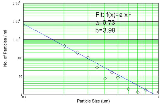
Figure 3: Particle size distribution of a “clean” sample.
