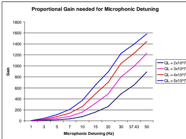
Figure 1: Proportional gain needed to compensate for microphonic detuning.
