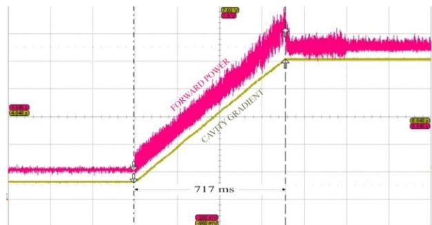
Figure 3: Graph of gradient and forward power as RF is turned on.
