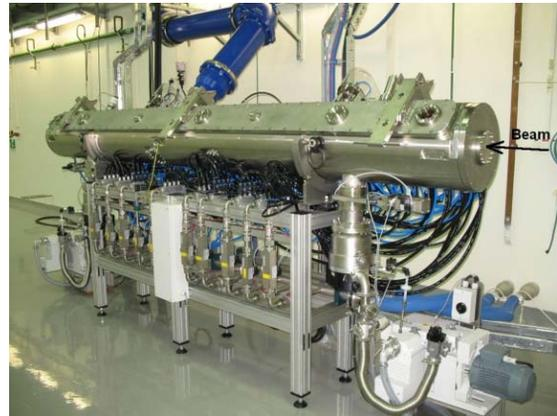
Figure 3: The RFQ as installed at Soreq. The 9” RF line, water pipes and vacuum pumps are also seen.
