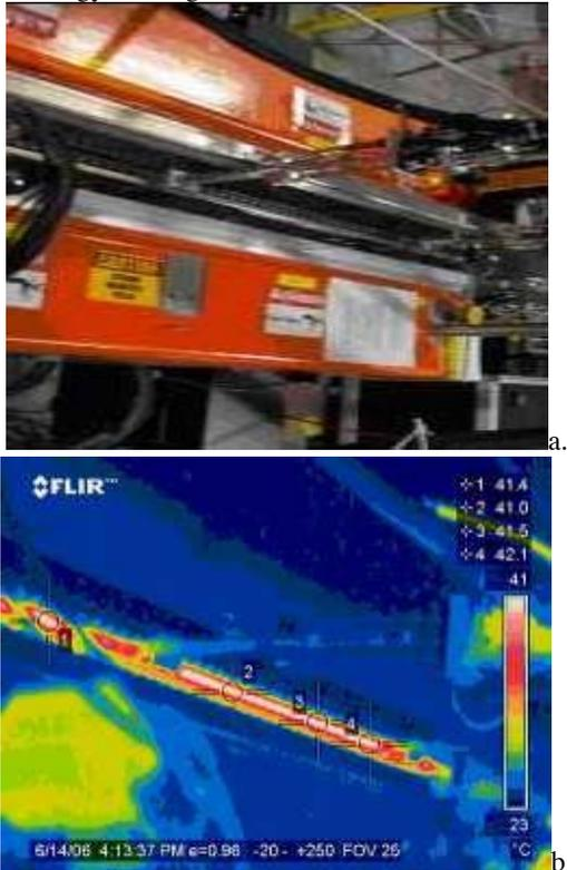
Figure 3. Visible (a) and infrared (b) images of the wiggler vacuum chamber showing strong resistive wall heating. The hottest part of the chamber is on the side hidden by the wiggler.
