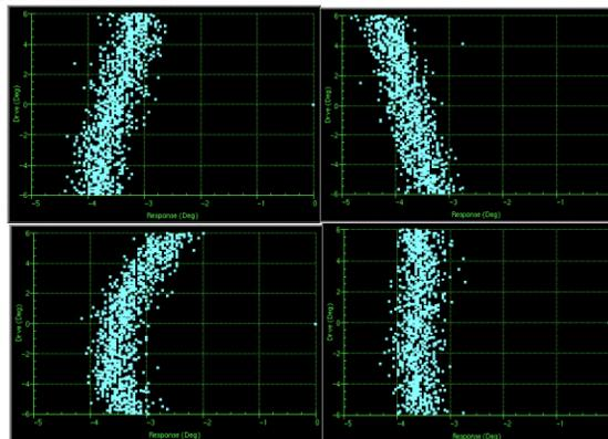
Figure 1. Input phase to linac vs. phase at the wiggler for the IR upgrade. The upper left image is with trim quadrupoles too strong. Upper right is with trim quads too weak. Lower left is with mispowered sextupoles, and lower right is properly set to produce maximum compression.
