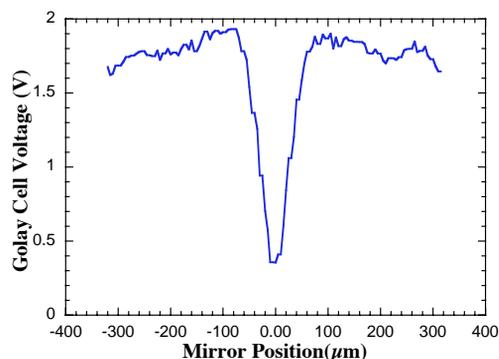
Figure 2. Coherent Optical Transition Radiation interferometer scan for typical operation. This scan indicates an *rms* bunch length of less than 150 fsec.
