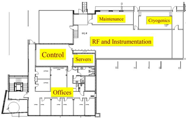
Figure 1: Layout of the top floor of the SARAF building. The Accelerator is located below the Maintenance and Cryogenics halls. The Targets Hall is further to the right.
