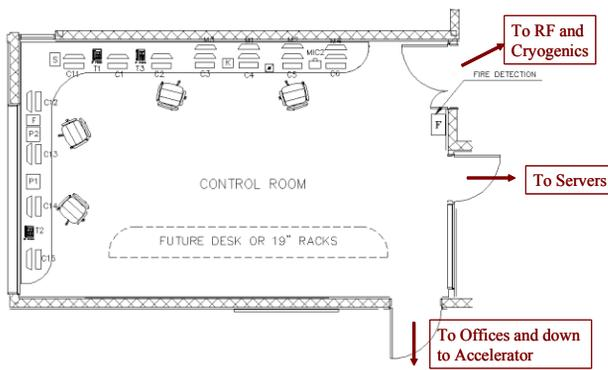
Figure 2: Layout of the MCR.
