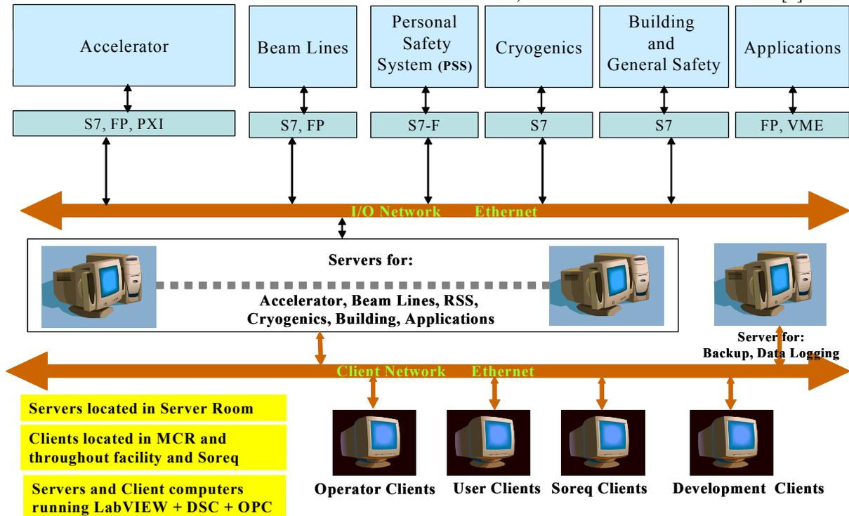
Figure 3: The architecture of the SARAF Main Control System.
