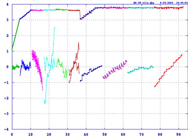
Figure 4:  $E_0$  in MV/m (upper) and tilt sensitivity in %/MHz (lower) versus accelerating-gap longitudinal position  $z$  (m). Design  $E_0$  is in red over the entire length. Measured  $E_0$  for each structure (in various colors) covers up most plotted design values.
