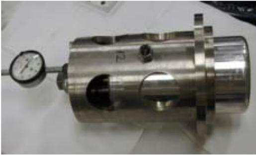
Figure 2: An adjustable aluminum slug tuner.
