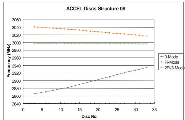
Figure 2: RF measurement of CLIC structure half cells.
