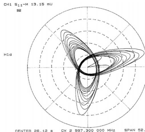
Figure 3: Bead pull measurement of a CLIC structure.
