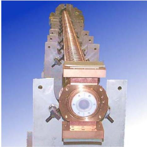
Figure 4: 5.2 m long S-Linac structure ready for delivery.
