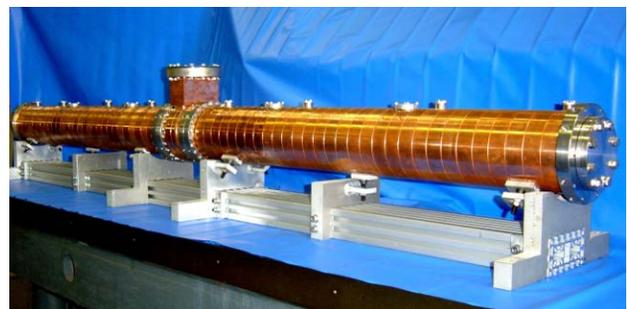
Figure 7: Complete brazed and assembled 2 m long MAMI-C 2.45 GHz structure.
