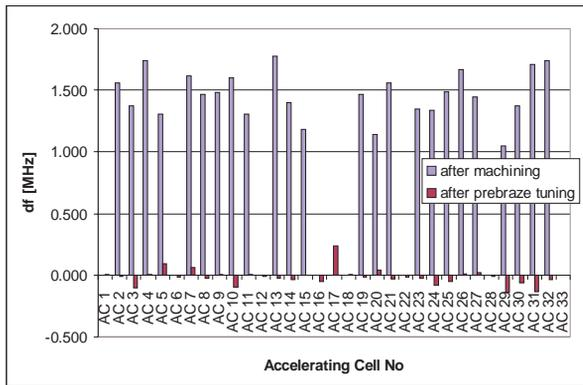
Figure 8: Frequency difference to target frequency before and after pre-braze tuning.
