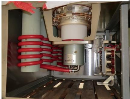
Figure 7: One of both tetrodes TH537 in anode down configuration. At the tube socket one sees the screen grid capacitor (500 nF) to ground unwanted RF currents. To the right there is the coupling capacitor and the contact tab to the cavity bus bar.
