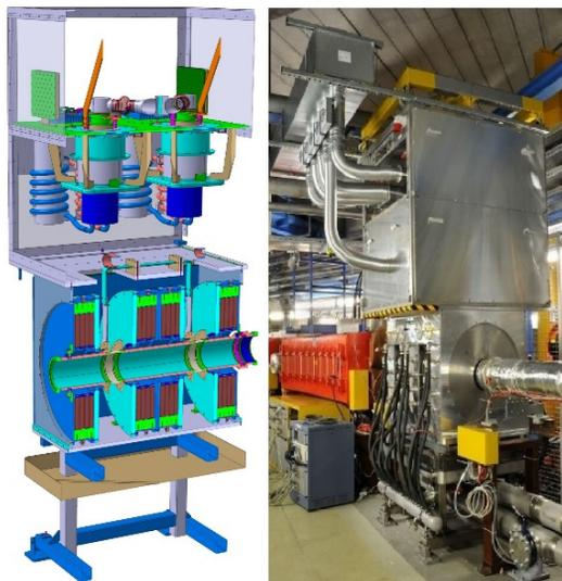
Figure 1: The picture to the left shows one unit of the  $h=2$  cavity and power amplifier arrangement already installed in the synchrotron ring. The picture to the right shows a cross-section of the cavity with its MA-cores and ceramic gaps at the bottom and the power amplifier with its two tetrodes on top.
