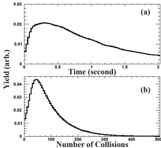
Figure 4: Resulting plots for (a) a  $^8\text{Li}$  release curve with one shot of a 100-MeV proton at  $t = 0$  and (b) the number of collisions of atoms with wall within a surface ionizer.
