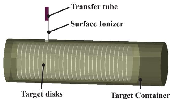
Figure 1: Three-dimensional rendering of four parts, which are directly related to the production of radioactive ions, of the present target-ion-source design in Geant4.
