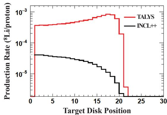
Figure 2: Simulated distributions of  $^8\text{Li}$  nuclei among BeO target disks inside the TIS. The incident beam is a 100-MeV protons with a uniform profile. The two production curves are obtained with cross sections calculated in the Liege intranuclear cascade model and TALYS.
