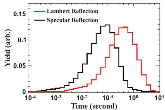
Figure 3: Time distribution of effusive flows of neutral  $^8\text{Li}$  atoms in pure (black) specular and (red) Lambert reflection modes. In above plots, diffusion is not considered and observed delay results entirely from effusion. The mean values for specular and Lambert reflections correspond to 51 ms and 290 ms, respectively.
