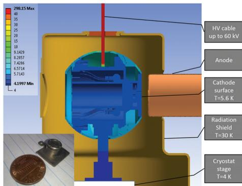
Figure 1: Thermal simulations have been performed using ANSYS®. Results indicate that a few K can be achieved at the cathode surface. The inset shows the new photocathode holder derived from the Scienta Omicron flag style.
