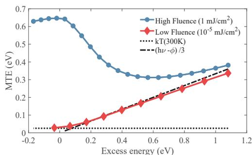
Figure 4: MTE calculated based on time evolving occupation function for different laser fluence. At low fluence, the result agrees with conventional three step model prediction while high fluence result shows non-monotonic behavior due to multi-photon absorption.
