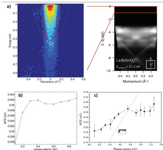
Figure 2: A) Measured band structure of the La:BaSnO<sub>3</sub>; B) Predicted MTEs from the measured band structure; C) Measurements of MTEs as function of photon energy.
