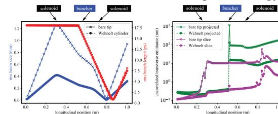
Figure 3: Plots showing the effect of a focusing Wehnelt electrode on a cathode with a field-enhancing tip. The left plot shows the beam size and bunch length the one on the right shows the emittance as a function of the position of the beam on the beamline (bunch charge is 11 fC).
