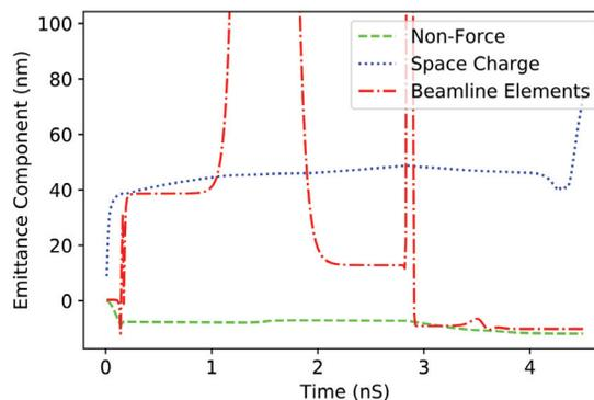
Figure 6: Emittance components along a highly optimized ultrafast electron diffraction beamline. The space charge component's large contribution to the final emittance suggests that it is the limiting factor in this system.
