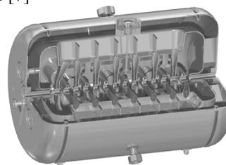
Figure 2: Sectional drawing of the 15-gap demonstrator CH-cavity (CH0).
