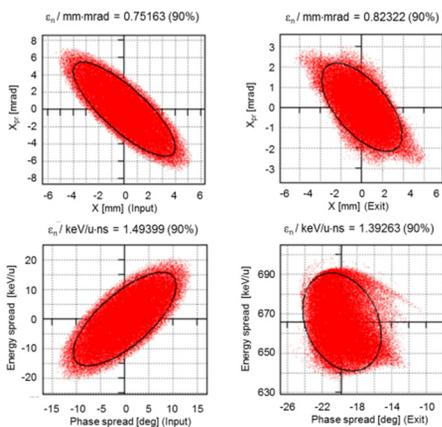
Figure 4: Phase space portraits applying an advanced Linac layout; top:  $x - x'$ , bottom:  $\Delta\phi - \Delta W$ , left: CM1-Input (emittance size as at HLI), right: Output of CM4 [20].
