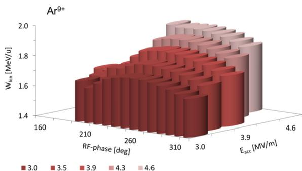
Figure 5: 2D-scan of Ar<sup>9+</sup>-beam energy versus accelerating gradient and RF-phase [21].
