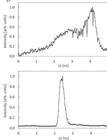
Figure 7: Bunch shape of Ar<sup>9+</sup>-beam at 1.366 MeVu (top) and fully matched at 1.85 MeV/u (down) [21].
