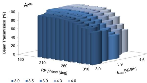
Figure 6: 2D-scan of Ar<sup>9+</sup>-beam transmission versus accelerating gradient and RF-phase [21].
