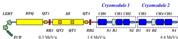
Figure 3: Advanced layout with three sc CH-cavities per cryomodule (two of four cryomodules are shown). Captions: QT = Quadrupole Triplet, RB = Rebuncher, S = Solenoid, B = 2-Gap-Buncher, D = Diagnostics.
