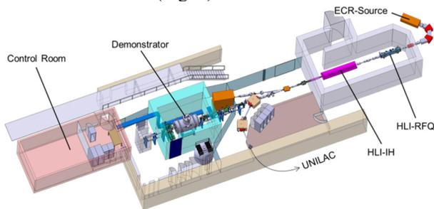
Figure 1: CH-cavity test environment at GSI.
