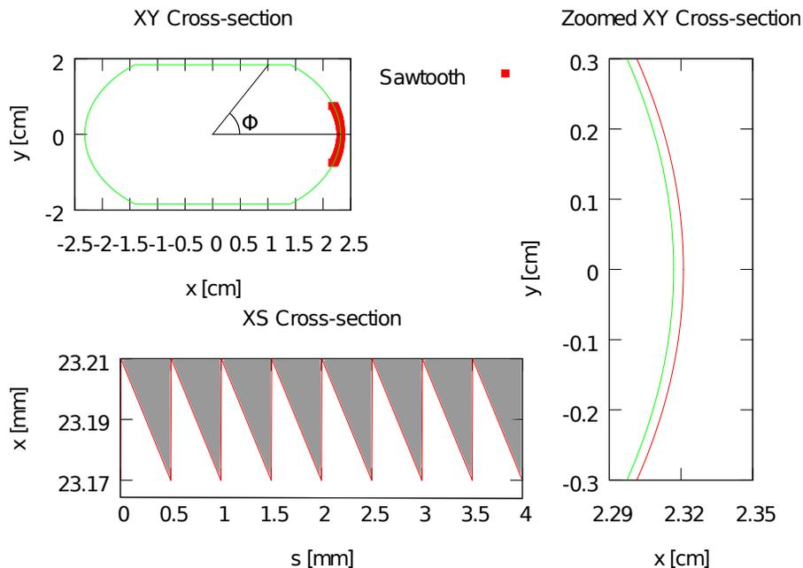
Figure 1: Synrad3D model of the LHC beam-screen design. (a)  $xy$  beam-screen cross section, (b) enlarged view of the sawtooth portion of the  $xy$  cross section, (c)  $xs$  cross section. A beam moving towards the positive  $s$  direction will see an inverted sawtooth; a beam moving towards negative  $s$  will witness the correct form of the sawtooth. [4]
