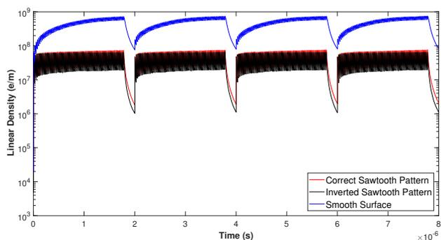
Figure 3: Electron linear density for a SEY = 1.3 and for a smooth chamber (blue curve), a sawtooth pattern correctly oriented (red curve) and an inverted-orientation sawtooth pattern (black curve).
