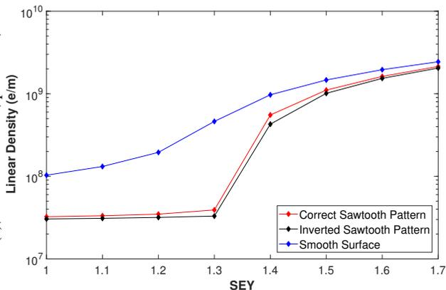
Figure 4: Average linear density as a function of SEY for three vacuum surfaces: smooth chamber (blue curve), correctly oriented sawtooth (red curve), and inverted sawtooth (black curve).
