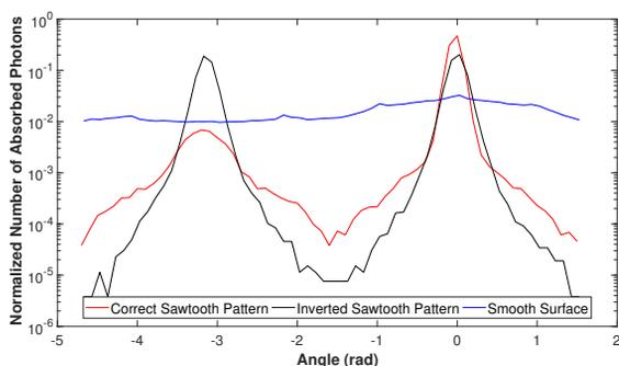
Figure 2: Simulated azimuthal distribution (integral normalized to unity) of absorbed photons without (blue curve) and with a sawtooth (red curve) and with an inverted sawtooth (black curve) chamber. [4]
