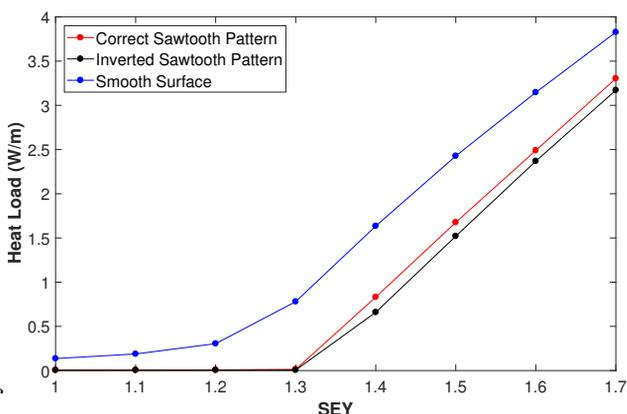
Figure 5: Average heat load as a function of secondary emission yield (SEY) for three vacuum surfaces: smooth chamber (blue curve), correctly oriented sawtooth (red curve) and sawtooth with inverted orientation (black curve).
