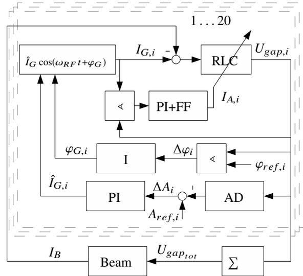
Figure 1: Block diagram of individual cavities with their control loops and beam dynamics.
