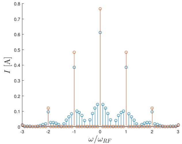
Figure 2: Fourier coefficients of the revolving bunch train in the case of eight of ten filled buckets (blue) and ten out of ten filled buckets (red).
