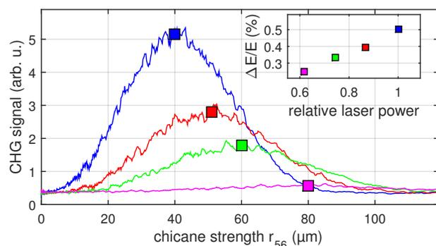
Figure 3: CHG signal versus chicane strength  $r_{56}$  for different laser pulse energies. Squares: Maximum signal. Top right: Corresponding relative modulation amplitudes  $\Delta E/E$  for different laser pulse energies.
