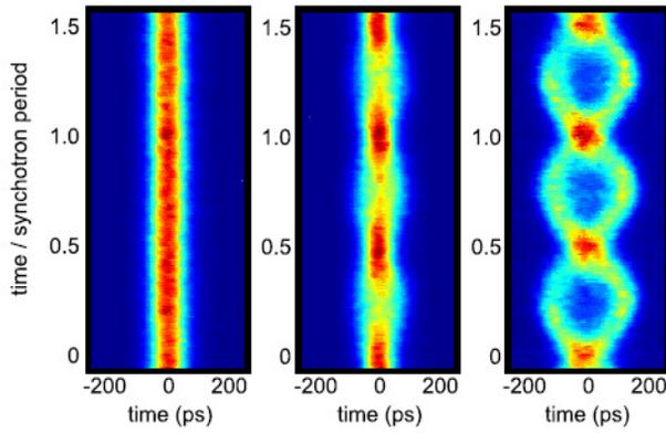
Figure 4: Streak camera images showing the evolution of the longitudinal bunch profile (horizontal axis) over 1.5 synchrotron periods (vertical axis) without RF phase modulation (left) and with RF phase modulation with increasing amplitude (center and right).
