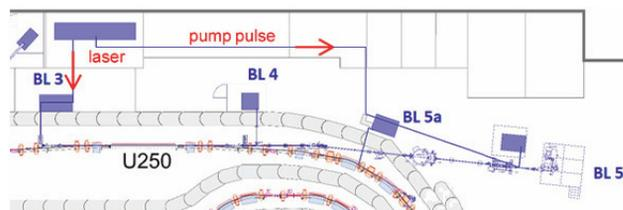
Figure 2: The short-pulse facility in the northern part of DELTA comprises a laser laboratory, the seeding beamline BL 3, the electromagnetic undulator U250, the diagnostics beamline BL 4, the VUV beamline BL 5, and the THz beamline BL 5a.
