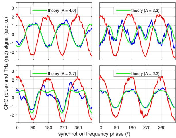
Figure 6: Laser-induced THz (red) and CHG (blue) signals (mean values subtracted) under the influence of an RF phase modulation versus the synchrotron frequency phase and theoretical CHG signals (green, from Fig. 5) for different energy modulation amplitudes  $A$ .
