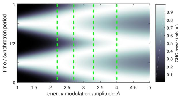
Figure 5: Normalized CHG power as function of the energy modulation amplitude  $A$  and time while  $s$  (see Eq. (5)) oscillates twice per synchrotron period due to RF phase modulation. Here,  $s$  oscillates between 0.7 and 1.3 and is smallest at  $t = 0$ . Curves used in Fig. 6 are indicated in green.
