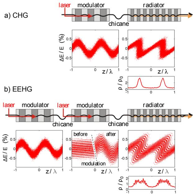
Figure 1: Magnetic setups for CHG (a) and EEHG (b), corresponding longitudinal phase space distributions and the final longitudinal charge density.
