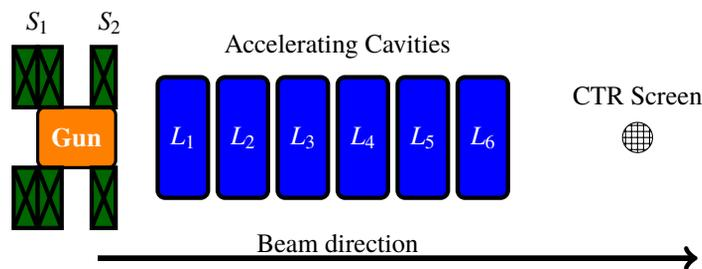
Figure 2: Beam line layout at the AWA.
