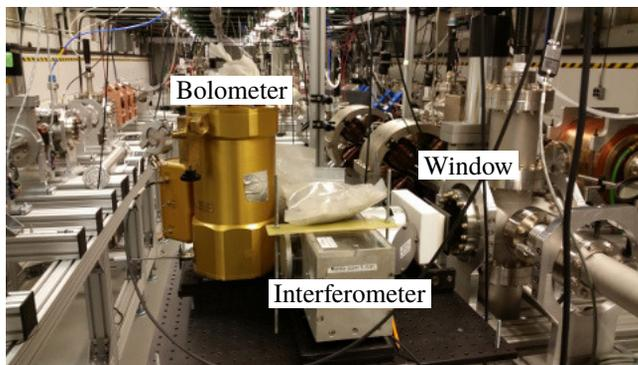
Figure 3: IR labs bolometer and MI interferometer used in the experiment to capture CTR light as it exited a window on the beam line.
