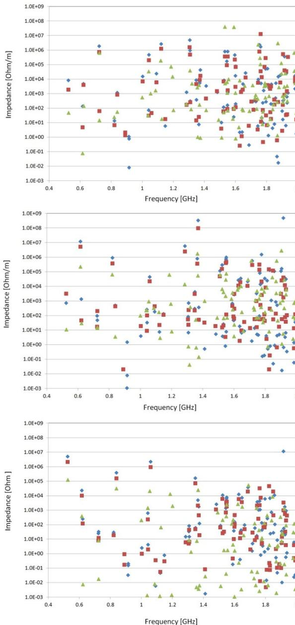
Figure 4: Comparison of deflection (top), vertical (middle), and longitudinal (bottom) impedance with different damping schemes. Each plot has magnetic couplers tip at port opening (blue diamond), 10 mm penetrated into cavity (red square), and electric couplers 10 mm penetrated into cavity (green triangle).
