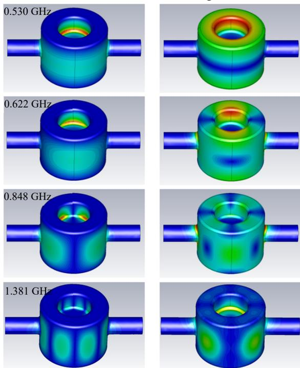
Figure 2: Typical HOM field distributions of the DQWCC with electric field on the left, and magnetic field on the right.
