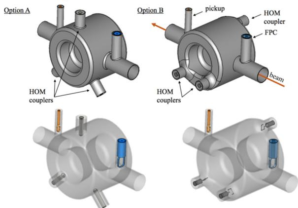
Figure 3: Electric (left) and magnetic (right) coupling of the HOMs.
