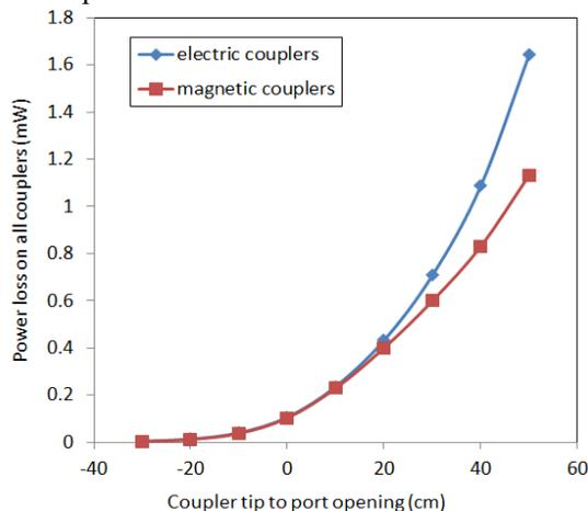
Figure 5: Comparison of power loss on all couplers at various penetrations between electric and magnetic coupling. Positive distance defined as couplers penetrate into cavity.
