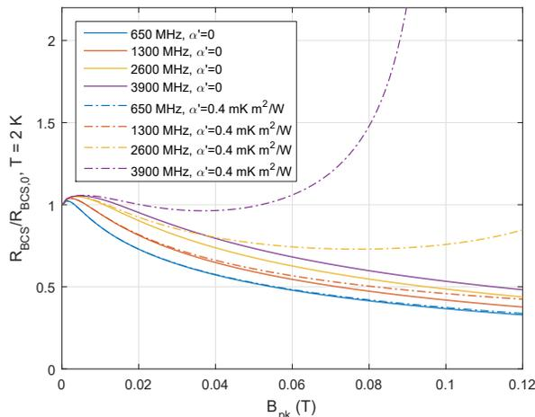
Figure 5: Theoretical predictions of the anti-Q-slope at 650 MHz, 1.3 GHz, 2.6 GHz, and 3.9 GHz, for  $\alpha' = 0$  and  $\alpha' = 0.4 \text{ mK m}^2/\text{W}$ , at 2 K.
