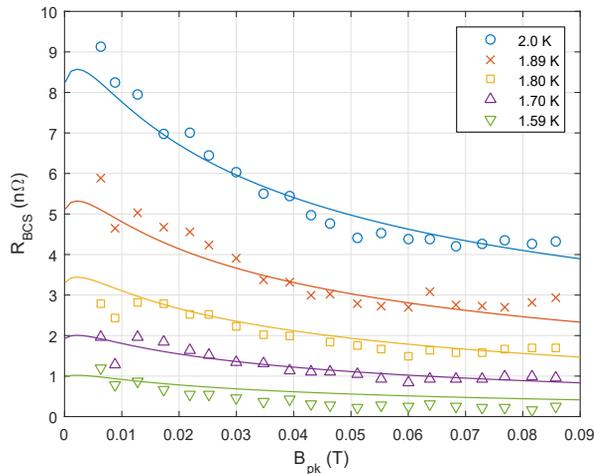
Figure 2: Field-dependent BCS surface resistance  $R_{\text{BCS}}$  data for the 160° C-doped single-cell cavity, with theoretical fit results. Theoretical curves correspond to  $\alpha' = 0.11 \text{ mK m}^2/\text{W}$ .
