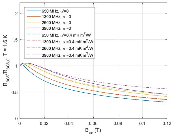
Figure 4: Theoretical predictions of the anti-Q-slope at 650 MHz, 1.3 GHz, 2.6 GHz, and 3.9 GHz, for  $\alpha' = 0$  and  $\alpha' = 0.4 \text{ mK m}^2/\text{W}$ , at 1.6 K.
