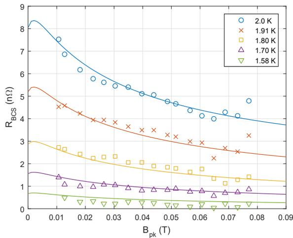
Figure 1: Field-dependent BCS surface resistance  $R_{\text{BCS}}$  data for the 160° C-doped nine-cell cavity, with theoretical fit results. Theoretical curves correspond to  $\alpha' = 0.19 \text{ mK m}^2/\text{W}$ .
