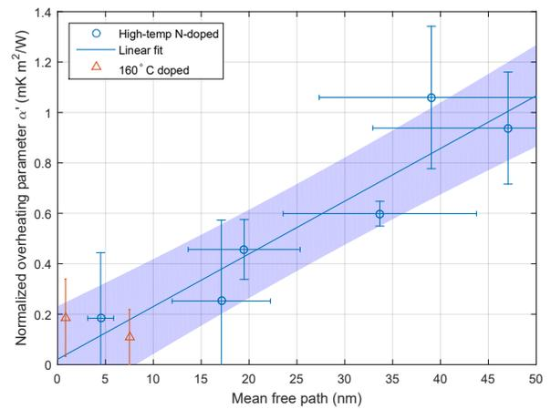
Figure 3: Normalized overheating parameter  $\alpha'$  as a function of mean free path  $\ell$ . High-temperature nitrogen-doped and fit originally published in reference [5]; new data for cavities doped at 160° C is displayed here over the original plot.
