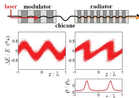
Figure 1: Sketch of the short-pulse scheme CHG with the electron distribution in phase space (relative energy deviation  $\Delta E/E$  versus longitudinal coordinate  $z$  in units of the laser wavelength  $\lambda$ ) and electron density  $\rho(z/\lambda)$ .
