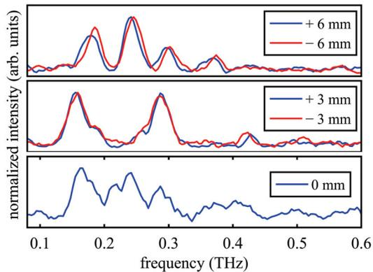
Figure 5: Sub-THz spectra one turn after the interaction between electrons and two laser pulses separated by 0,  $\pm 3$ , and  $\pm 6$  mm. The symmetry with respect to the sign of the separation confirms the zero-delay assumption.
