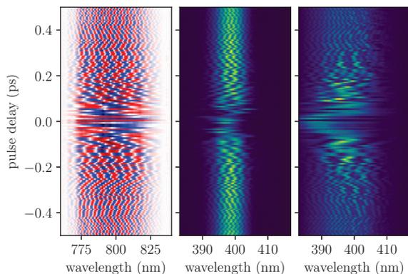
Figure 4: Under variation of the delay between two laser pulses, their spectral interference pattern (left) and interference of 400-nm CHG radiation are shown for two distinctly different cases, a small chirp precompensating the effect of propagation through the vacuum window (center, pulse length 50 fs) and a larger chirp (right, pulse length 90 fs).
