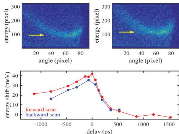
Figure 3: Raw data from the DLD at pump-probe delay 1500 ps (top left) and at 0 ps (top right) with an apparent energy shift of the Cu(111) surface state which depends on the delay (bottom). The difference between the forward and backward scan is consistent with an additional shift depending on the bunch current and thus on the CHG intensity.
