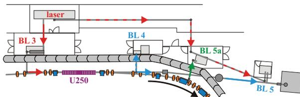
Figure 2: The short-pulse facility at DELTA comprising a laser system, a laser beamline (BL 3) guiding seed pulses to the undulator U250, a diagnostics beamline (BL 4), a soft-x-ray beamline (BL 5), and a THz beamline (BL 5a).
