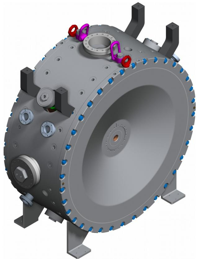
Figure 3: Technical design of CH cavity 1.
