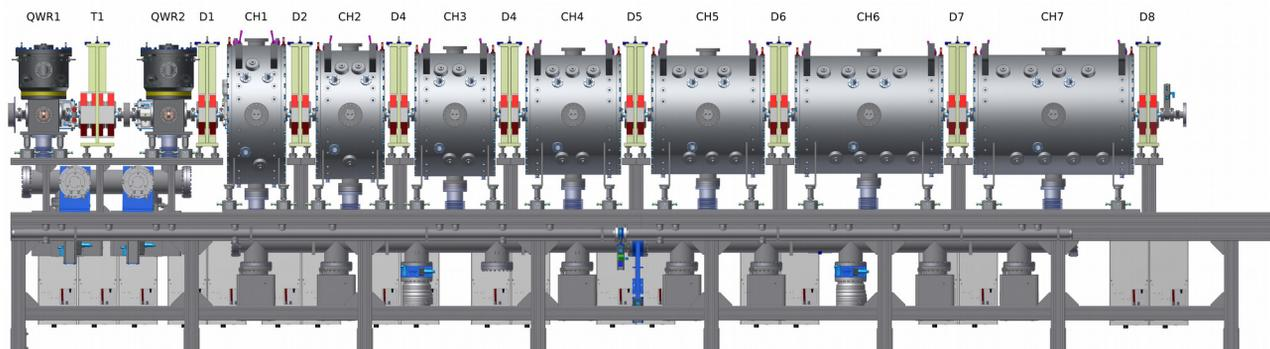
Figure 1: MYRRHA Injector construction scheme up to 5.9 MeV.
