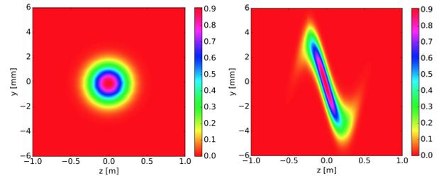
Figure 4: 2D gaussian beam in  $y$  and  $z$ , without (left) and with a kick corresponding to 6.8 MV (right).
