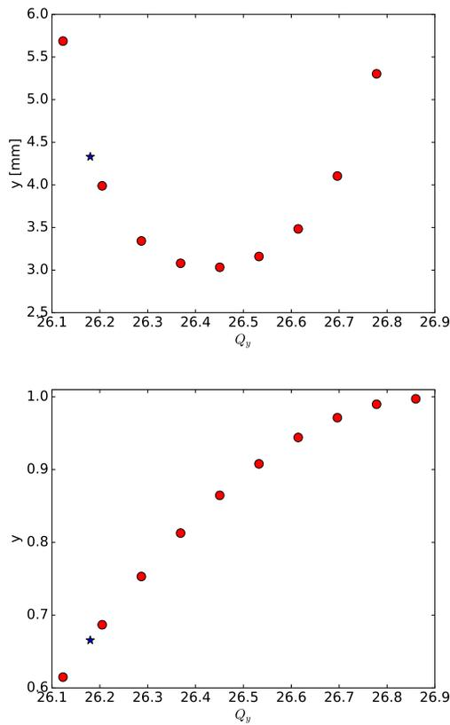
Figure 1: Absolute (top) and normalised (bottom) vertical CO offset at the HT monitor as a function of  $Q_y$ ; blue star: vertical operational tune (26.18).
