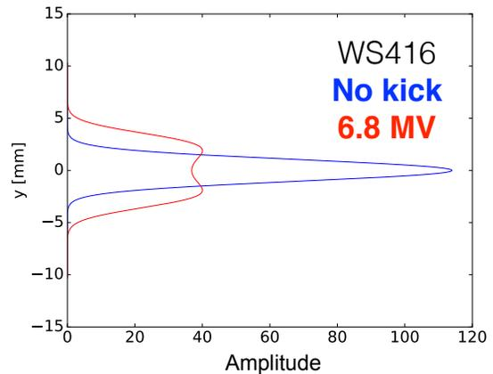
Figure 5: Vertical beam profile without (blue) and with a kick corresponding to 6.8 MV (red).
