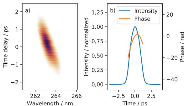
Figure 3: UV FROG pulse trace of the beam after the prism stretcher. The measured spectrogram is shown in panel a, with a clear tilt representing a frequency chirp in the pulse. In panel b, the reconstructed trace is plotted. The pulse duration is 1.3 ps FWHM and the chirp is evident as a quadratic phase curve.
