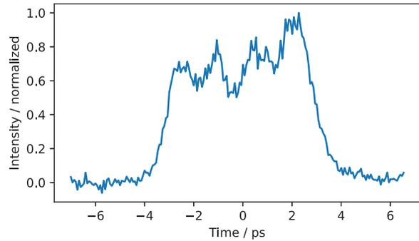
Figure 2: Cross correlation plot of four stacked pulses.
