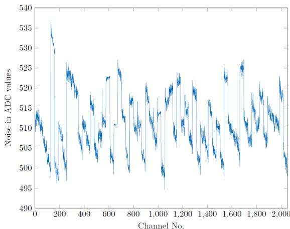
Figure 3: Example of the noise (mean of 4000 events in ADC values) per Channel of the R-type sensor.
