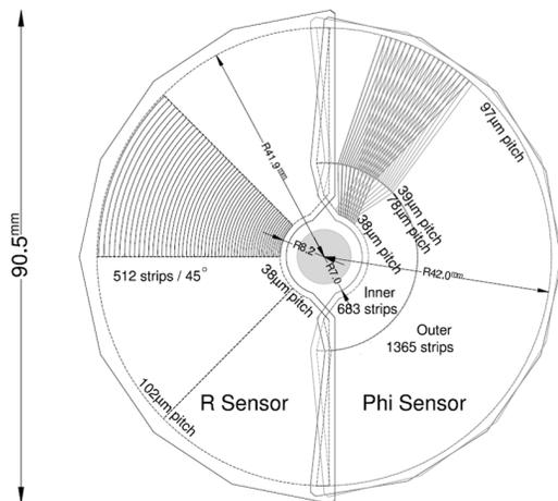
Figure 1: Sketch of the two VELO modules summarising the design of the R- and  $\phi$ -type sensor [3].
