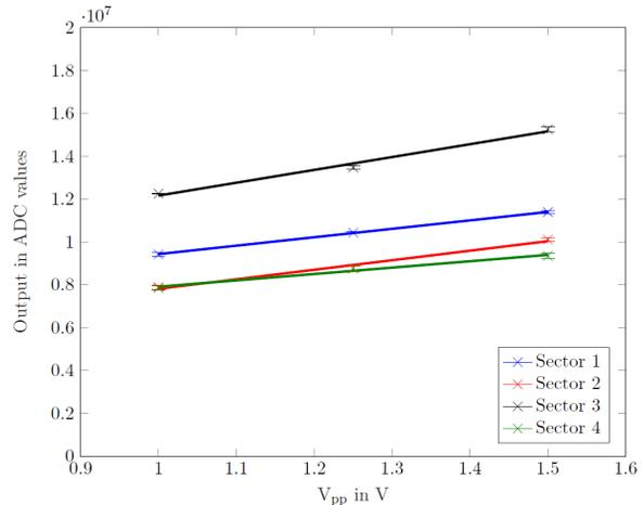
Figure 4: Output as the sum of 4000 events of VELO for three different Peak-to-peak voltages for the R-type sensor.
