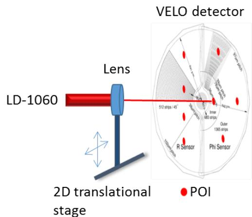
Figure 2: Setup of the LD-1060 to measure the output of the R-sensor and the  $\phi$ -sensor for different peak-to-peak voltages. The red dots indicate the points of interest (POI, not true to scale).
