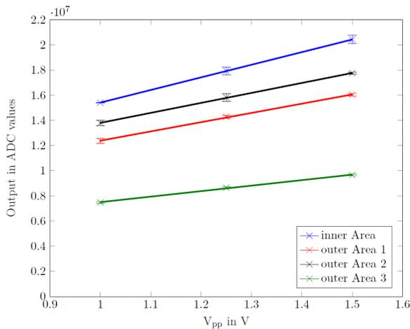
Figure 5: Output as the sum of 4000 events of the VELO for three different Peak-to-peak voltages for the  $\phi$ -type sensor.
