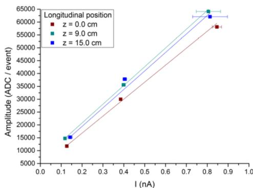
Figure 7: Average increase of the integrated ADC values in the  $\phi$ -sensor No. 76 per readout event versus the proton beam intensity measured by the FC [4].
