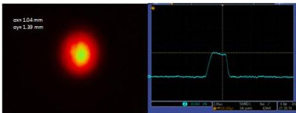
Figure 4: Output SCDTL4: (Left) Beam spot (Right) Pulse current on fast current transform.
