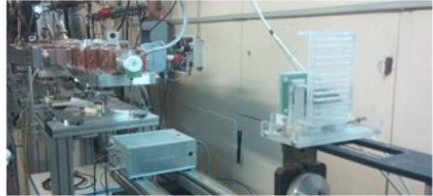
Figure 7: Irradiation setup of biological samples at 1 meter from the exit window.
