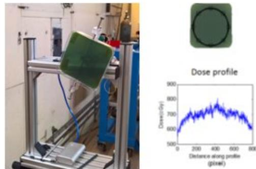
Figure 8: (Left): EBT3 film mounted on the target rotation system placed at 1.44 m from the accelerator exit (Right): Film analysis in a circle with 50.2 mm of radius.
