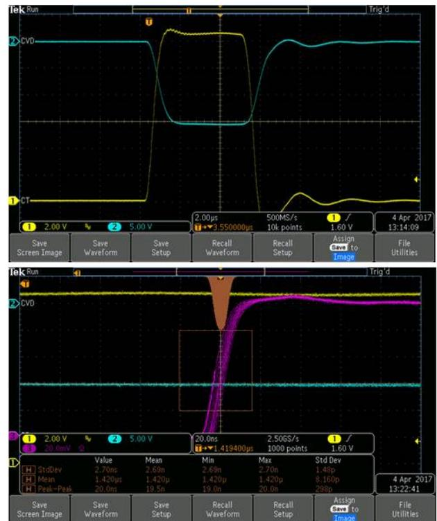
Figure 5: Scandinova K1 Modulator + TH2157A klystron test on water load. (Top): klystron voltage and current. (Bottom): klystron current jitter measurement.
