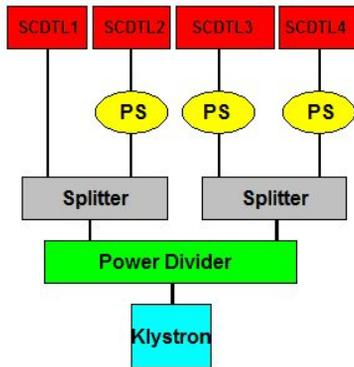
Figure 3: Schematic drawing of RF power distribution in the first section of TOP-IMPLART accelerator.
