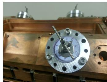
Figure 6: Slug tuner of the RFQ: 1 turn = 1 mm.
