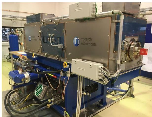
Figure 1: SIS100 Accelerating Cavity.
