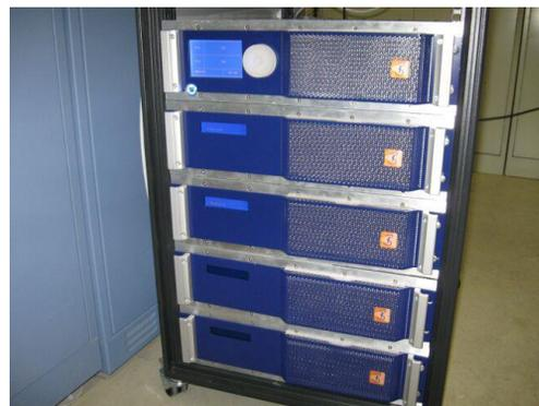
Figure 3: Modular solid-state power amplifier.
