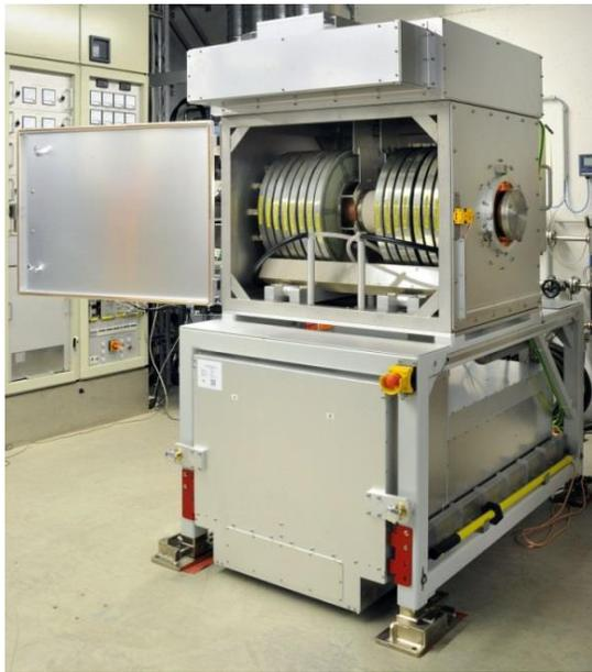
Figure 2: SIS100 Bunch Compressor Cavity.
